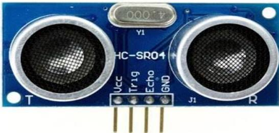
Gambar 4 Sensor Ultrasonic
