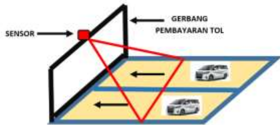
Gambar 4.2 Sensor dan Radio Frequency Identification (RFID) di Gerbang Tol Otomatis (GTO)
